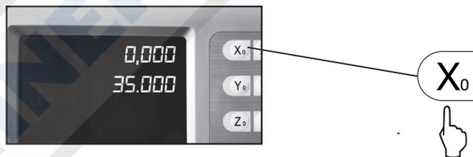
Step 2. Using the edge finder locate the edge at the other end of the work piece.
