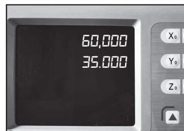
Step 3. Press **1/2** then **X** to half the "X" axis display value.
