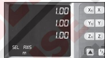
5. Set the resolution of Y axis: Z axis by repeating step 3-4.
