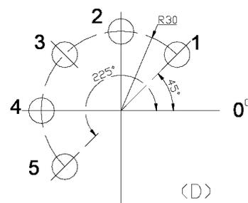
**Note:** If the ST.ANGLE equals the END.ANGLE, the holes are attributed equally around the whole circumference.
